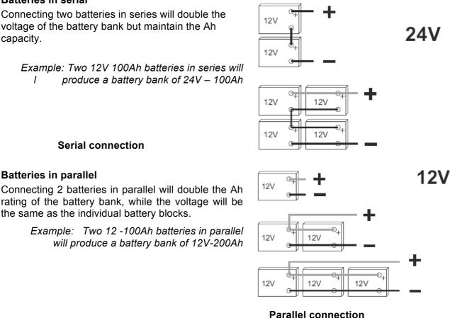
Example: Two 12V 100Ah batteries in series will produce a battery bank of 24V – 100Ah 1
