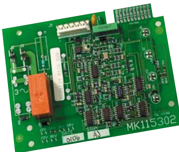
A printed circuit board with monitoring functions ensures safe charging.
